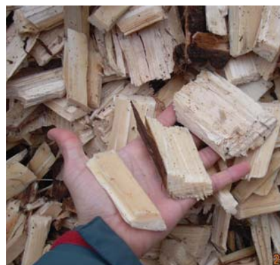
Chip sizes: 7.5cm (above), 2-3cm (below) and sawdust (bottom).
