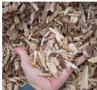
Chip sizes: 7.5cm (above), 2-3cm (below) and sawdust (bottom).
